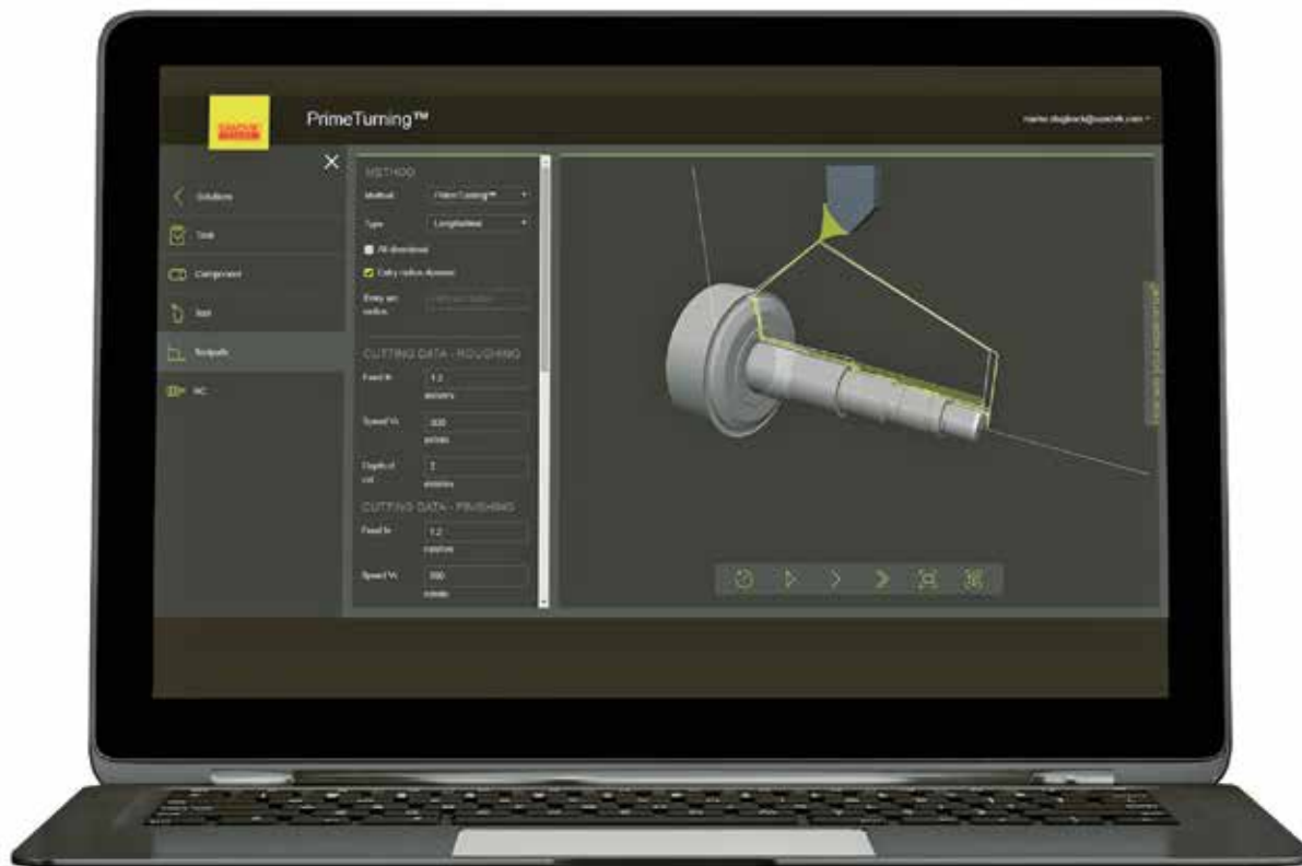
CoroPlus Tool Path enables efficient planning and programming of machining methods, such as PrimeTurning and OptiThreading
